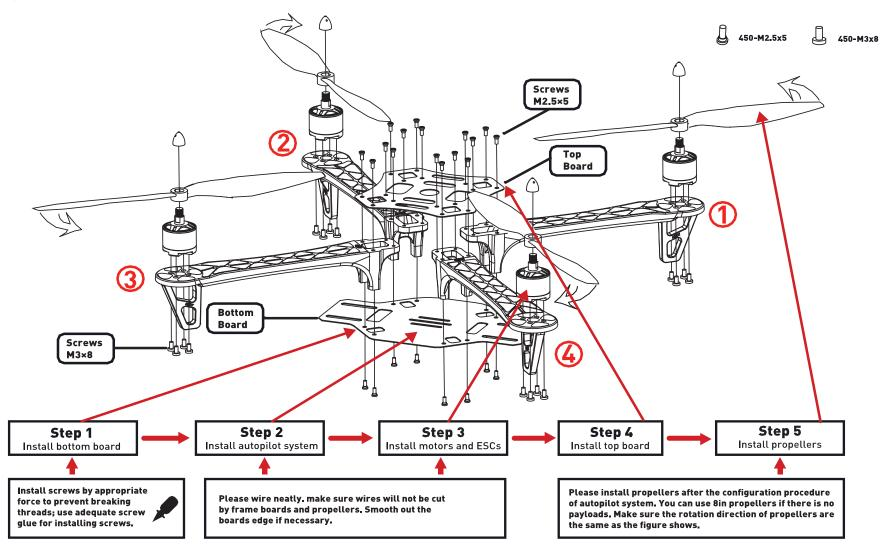
In up figure, arms ①, ② are front of craft; arms ③, ④ are back of craft. You'd better choose the same colour arms for the same direction. See from top, motors on arms ①, ③ rotate counter-clock wise, and use propellers 1045; motors on arms ②, ④ rotate clock wise, and use propellers 1045R.
