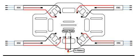
Please solder ESCs to bottom board as the up figure shows. Use any insulating method at all soldering spots. Make sure there is no short or open circuit. Make sure the side with bonding pads is upward.
