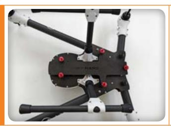
Screw the quick release nut on landing gear holder and slide legs into it.
