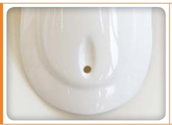
Drill a 8mm hole in your canopy and glue the grommet holder in place.
