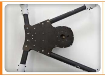
Remove the knuckles and mount the upper frame. Use M4\*40mm buttonhead in rear outer hole for fixing canopy standof.
