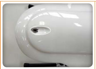
Mount the grommet into holder, fix the canopy with the body clip.
