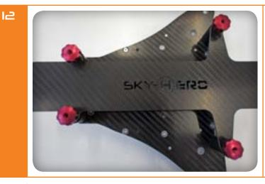
Mount your inertic plate. Screws used: M4 red knuckle
